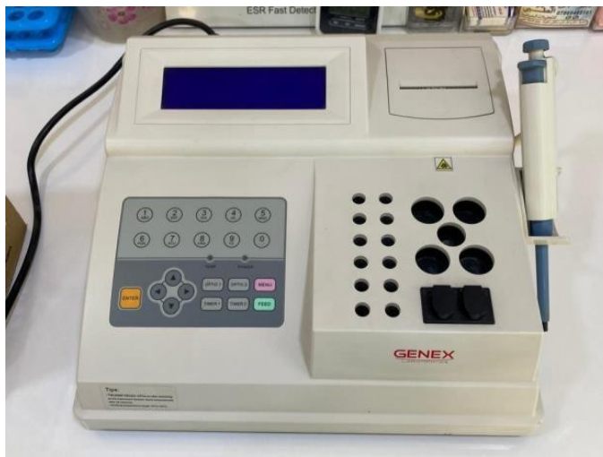
Figure 2. GENEX Thrombo semi-automated coagulation analyzer used for determination of PT, APTT, and fibrinogen
